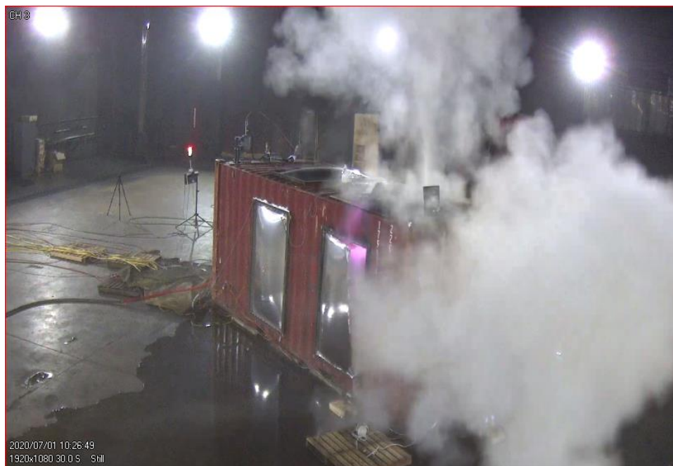
Figure 135 – Deflagration and side vent operation in Test 3 (test time 01:11:55).
