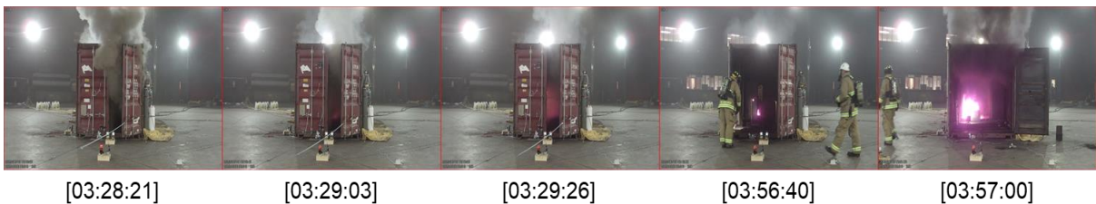
Figure 45 – Sequence of reignition during overhaul of Test 1 (test time 03:29:21 to 03:57:00).
