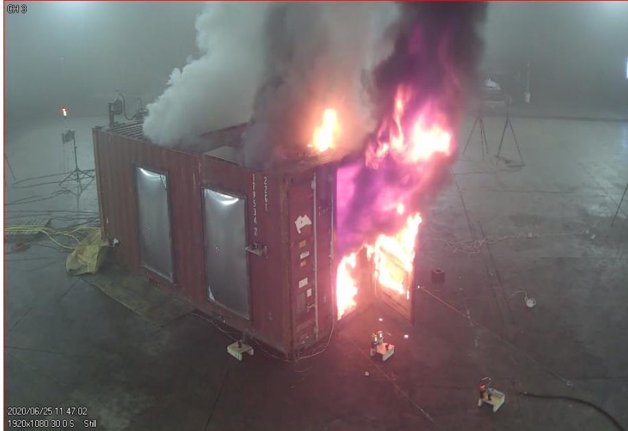
Figure 84 – Flaming of container contents after door opening in Test 2.
