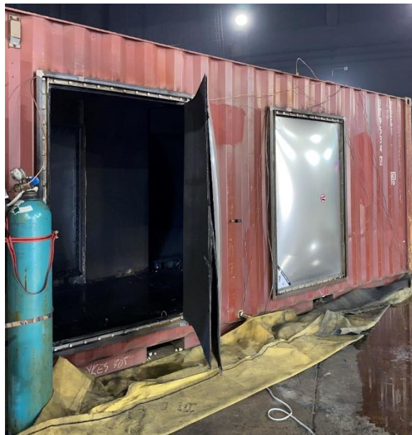
Figure 96 – Condition of deflagration vent after Test 2.
