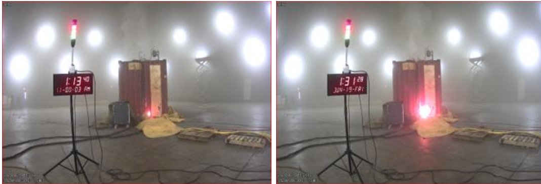
Figure 43 – Flaming outside the test container through cable conduit in Test 1.
