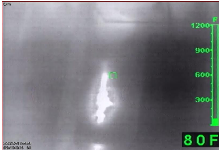
Figure 144 – Snapshot of thermal imaging camera facing the Initiating Unit suggesting additional off-gassing or flaming (test time 00:54:06).
