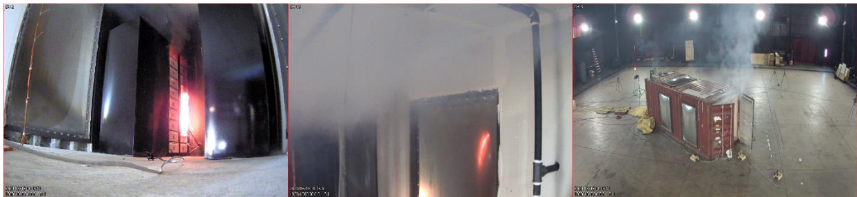
Figure 54 – Smoke layer condition upon activation of both smoke detectors in Test 1.
