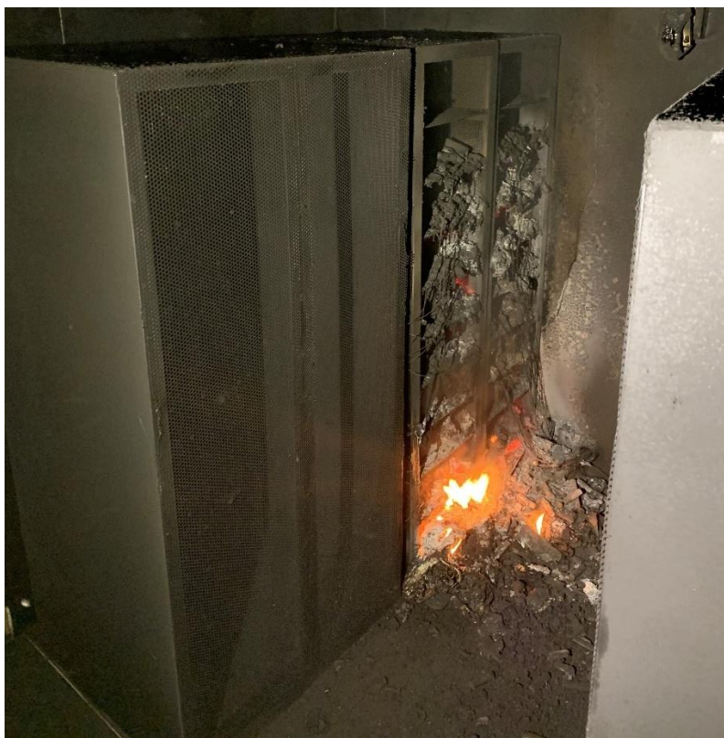
Figure 46 – Re-ignited fire observed during overhaul of Test 1 (four hours after test start).
