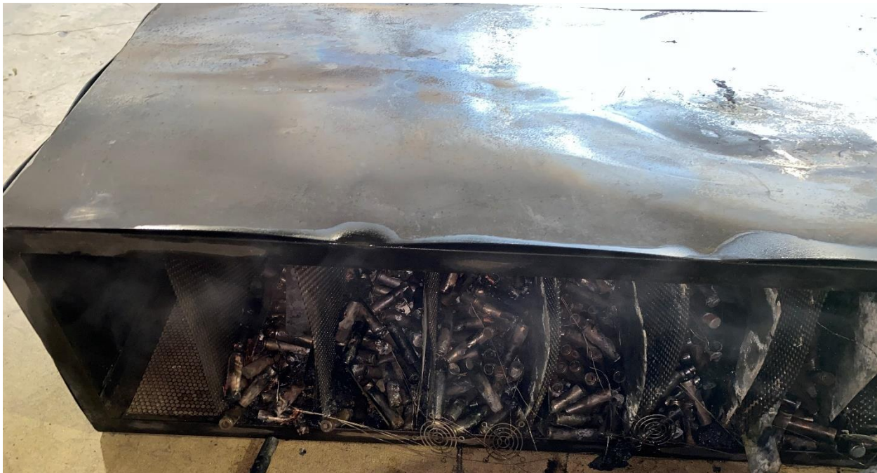
Figure 89 – Condition of Initiating Unit after Test 2.
