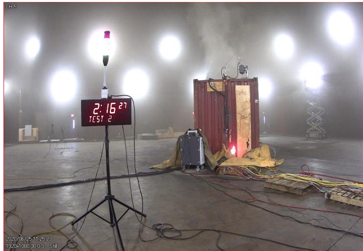
Figure 82 – Flaming observed intermittently through instrumentation opening in container wall in Test 2.
