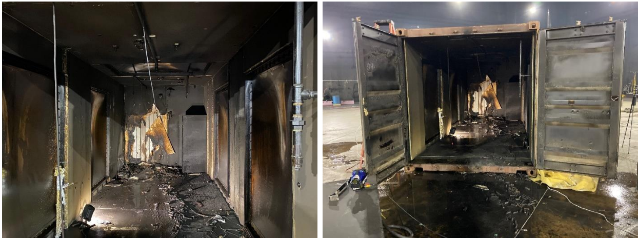
Figure 53 – Condition of container after Test 1 overhaul.
