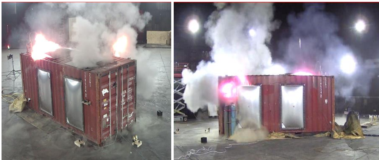
Figure 83 – Short duration flaming observed from deflagration vents.
