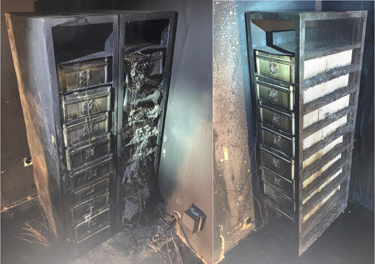
Figure 134 – Condition of Left Target Unit (left), Initiating Unit (left), and Front Target Unit (right) after Test 3.
