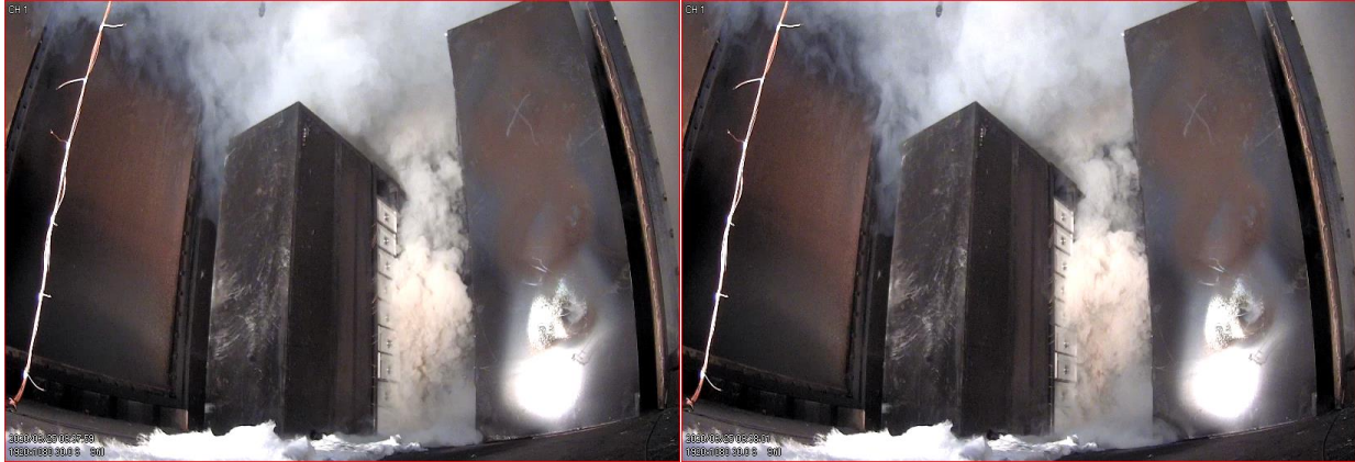
Figure 97 – Smoke layer condition upon activation of near (left) and far (right) smoke detectors in Test 2.
