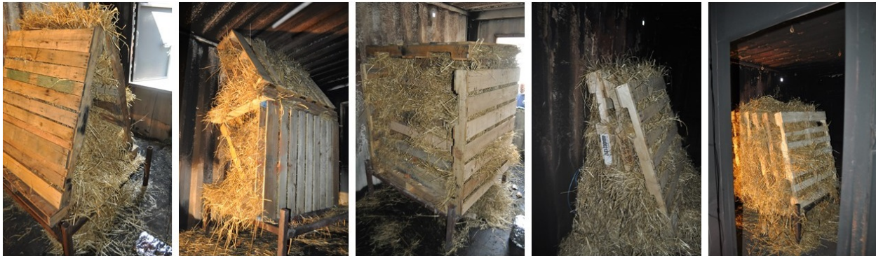
Figure 5.7: Images of 3 and 6 pallet configurations. From left to right: three pallet triangle, six pallet boxed-in triangle, six pallets stacked to form a platform, three pallet lean-to, and six pallet lean-to.
