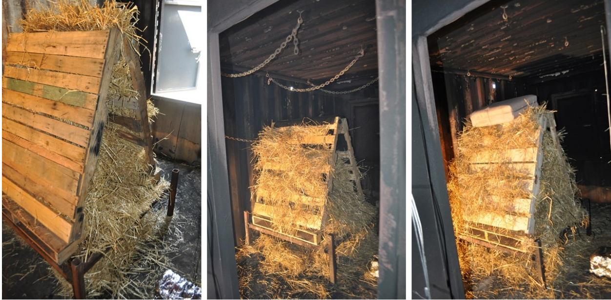
Figure 5.20: Three pallets and one bale of straw oriented in a triangle with no synthetic material (left), with tar paper (center), and with a polyurethane sofa cushion (right). 4.8 lbs (2.2 kg) of tar paper and 4.6 lbs (2.1 kg) of polyurethane foam were used in the fuel packages.
