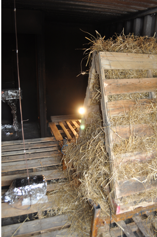
Figure 5.33: Fuel package with pallets on floor
