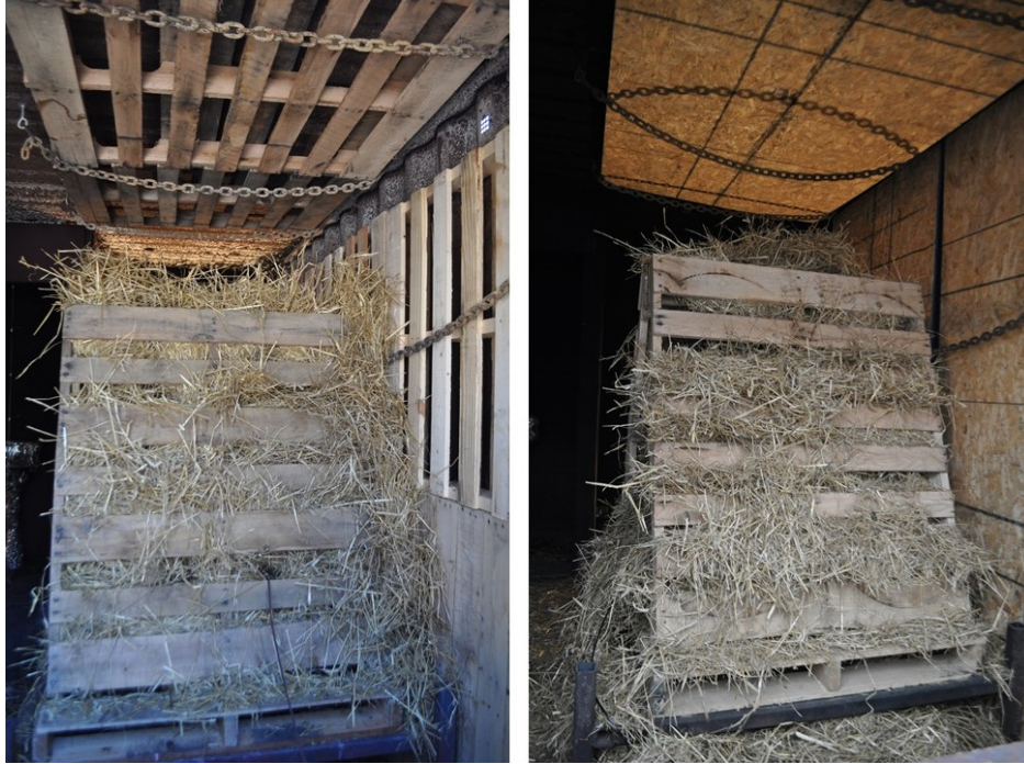
Figure 5.31: Fuel package with pallets on wall and ceiling (left) vs. OSB on wall and ceiling (right).
