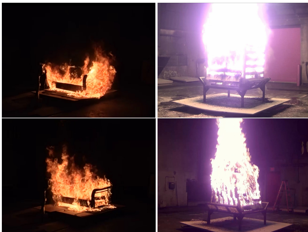
Figure 4.26: Images corresponding to the peak HRR for the upholstered sofa ignited in the center (top left) and right arm (bottom left) compared to wood-based training fuel packages of comparable peak HRRs. The center-ignition sofa had a peak free burn HRR of 3.47 MW which is comparable to the six pallet boxed-in triangle fuel load (top right) which had a peak HRR of 3.64 MW. The right-ignition sofa had a peak HRR of 3.72 MW, which is comparable to the six pallet lean-to (bottom right), which had a peak HRR of 3.21 MW. The error bars corresponding to each point indicate the uncertainty of the measurement.
