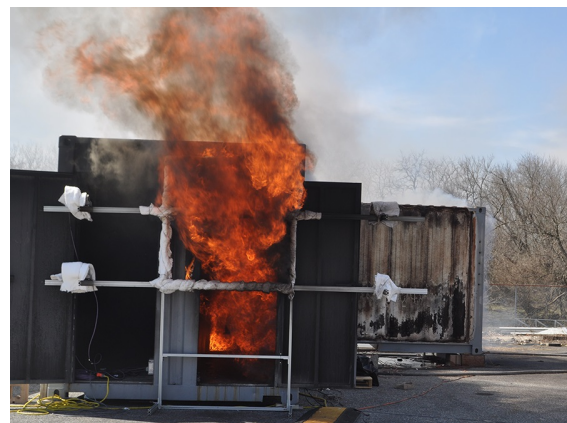
Figure 6.14: Heat flux at the level of a kneeling firefighter just outside the fire compartment (left) and still image from camera outside the hallway door at 410 s (right), demonstrating the effect of adding additional fuel to the hallway during a hallway and room burn in a container prop. The growth of the training fuel props was offset by 200 seconds to match the growth of the furnished room.
