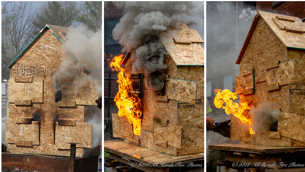
Figure 6.8: Scaled house burns demonstrating ventilation limited fire, from NFFF Fire Dynamics Boot Camp Howard County Maryland (left); neutral plane, from FireHouse Expo Aggressive Fire Control, Flow Path and VEIS Tactics class 2018 by All Hands Fire Photos (center); and flow path from FireHouse Expo Aggressive Fire Control, Flow Path and VEIS Tactics class 2018 by All Hands Fire Photos (right).
