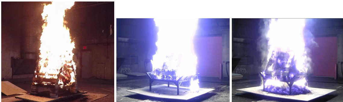
Figure 4.16: Visuals of three pallet fuel packages at the time of the peak free burn HRR. From top to bottom, left to right, the images show the 3P1S (2.05 MW), 3P1E (3.04 MW), and 3P2S (2.45 MW) fuel packages
