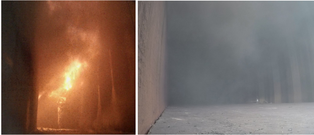
Figure 6.13: Difference in visible rollover with three pallets, one bale of straw, and three sheets of OSB in fire room with OSB on hallway ceiling (left) and without OSB on hallway ceiling (right)
