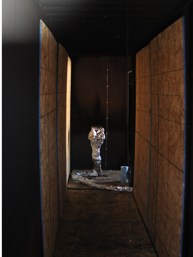
Figure 5.28: OSB on hallway walls for Experiment 4
