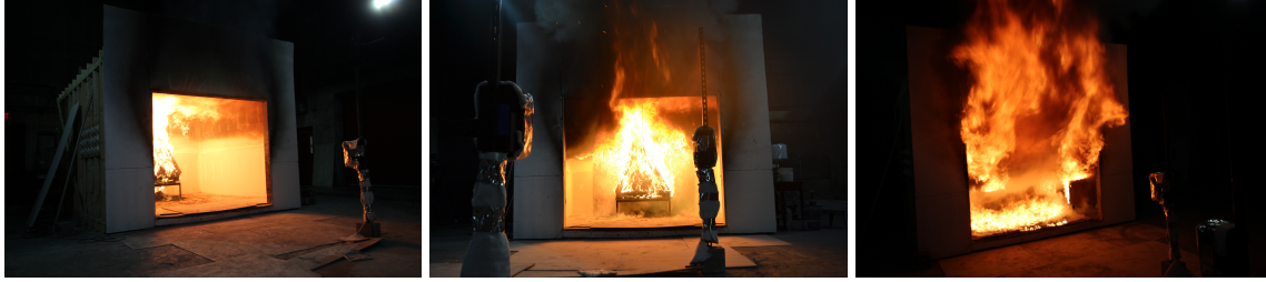
Figure 4.34: Comparison of peak burning conditions for 3P1S (left), 3P1SO (center), and furnished room (right).
