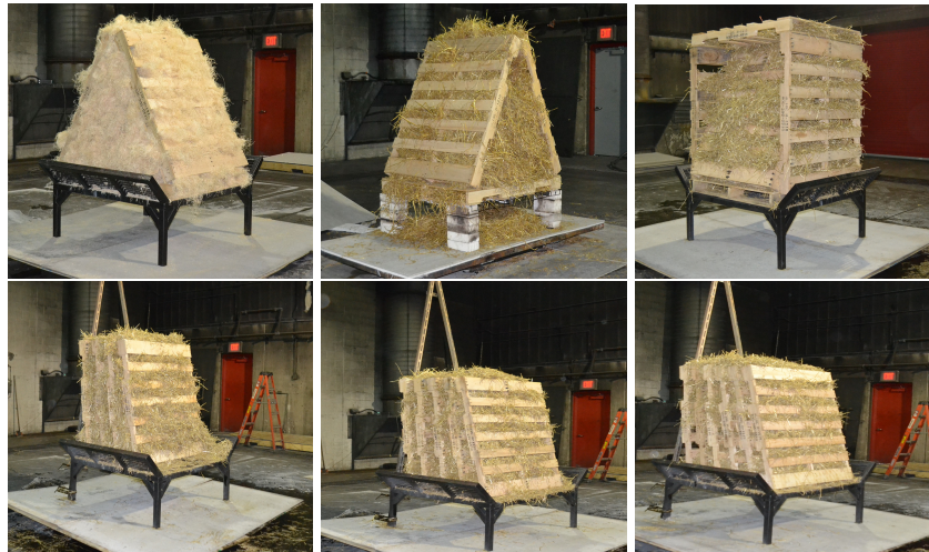
Figure 6.1: Characteristics of some common fuel packages. Less dense easily ignitable material surrounded by more dense longer burning duration fuels. 1 bale of excelsior with a 3 pallet triangle (top left), 1 bale of straw with a 3 pallet triangle (top middle), 1 bale of straw with a 3 pallet triangle and 3 pallet box (top right), 4 Pallets vertical with 1 bale of straw (bottom left), 5 pallets vertical with 1 bale of straw (bottom middle), 6 pallets vertical with 1 bale of straw (bottom right).
