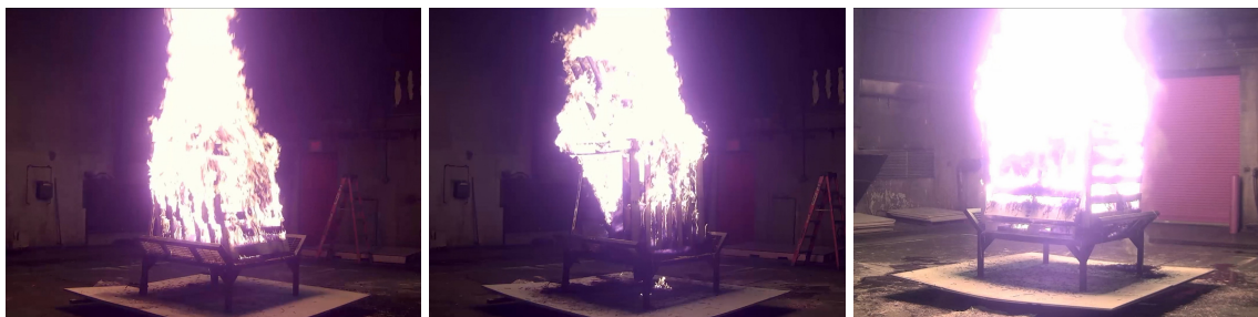
Figure 4.21: Visuals of fuel packages at the time of the peak free burn HRR. From left to right, the images show the 6P1S-V (3.19 MW), 6P1S-Fi (3.80 MW), and 6P1S-Ga (3.64 MW) fuel packages
