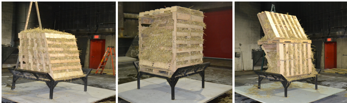
Figure 4.19: 6 Pallet Fuel Package Comparison. Each fuel package has 6 pallets and one bale of straw. Fuel packages shown are labeled 6P1S (left), 6PGa (center), and 6PFi (right)
