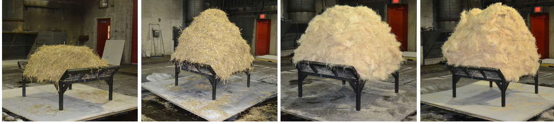
Figure 4.8: Images of fuel packages consisting of one (1S, top left) and two (2S, top right) bales of straw and one (1E, bottom left) and two (2E, bottom right) bales of excelsior.
