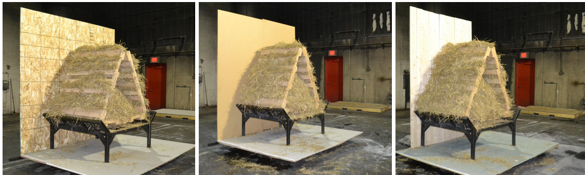
Figure 4.22: OSB (left), MDF (middle), and 1 in. x 6 in. dimensional lumber (right) fuel packages. Each fuel package has three pallets and one bale of straw in addition to the boards/lumber.
