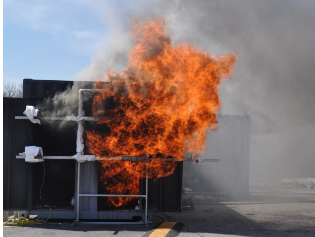
Figure 5.30: Fire venting from prop doorway in Experiment 4
