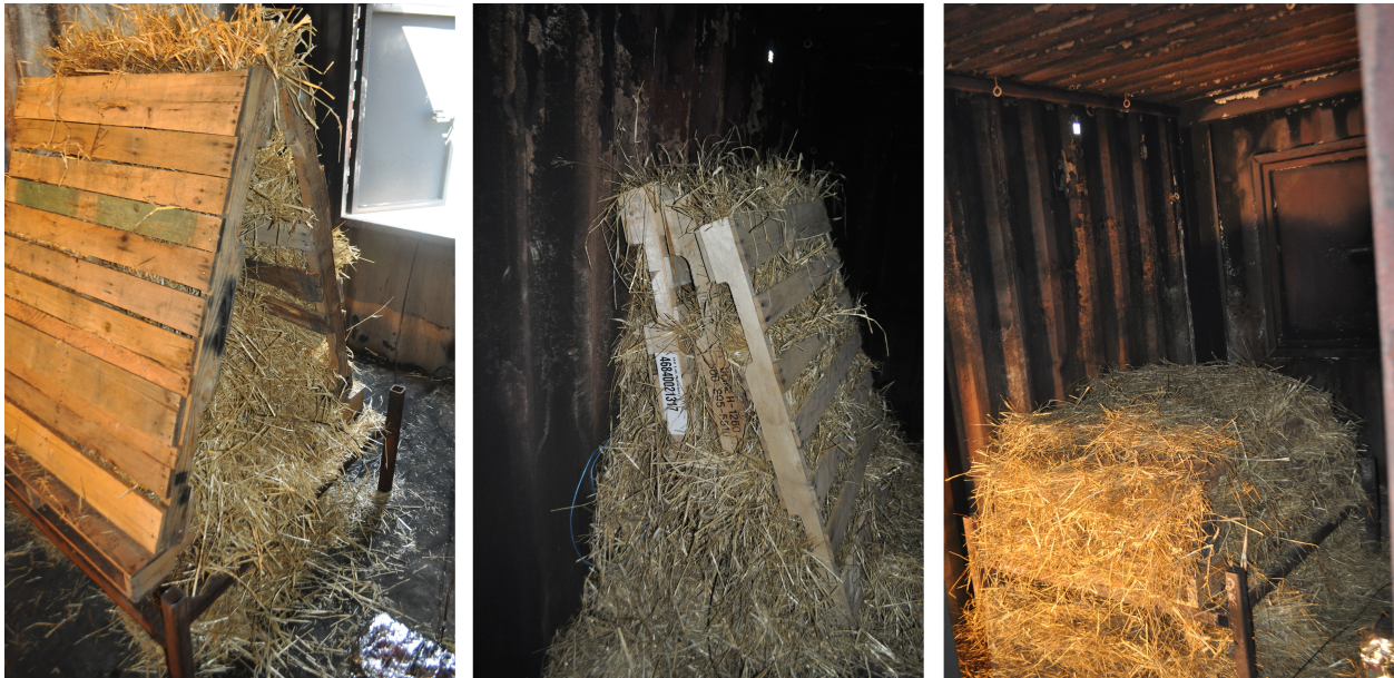
Figure 5.3: Three pallets and one bale of straw oriented in a triangle (left), a lean-to (middle), and horizontally stacked (right)
