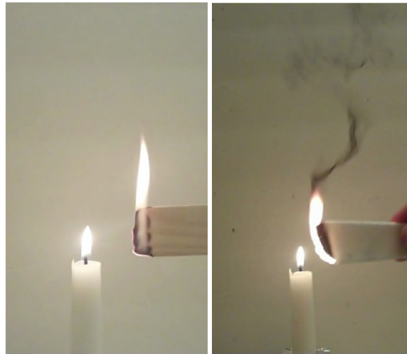
Figure 6.7: Candle demonstrations of fire dynamics principals. Wood fuels (left) and synthetic fuels (right).
