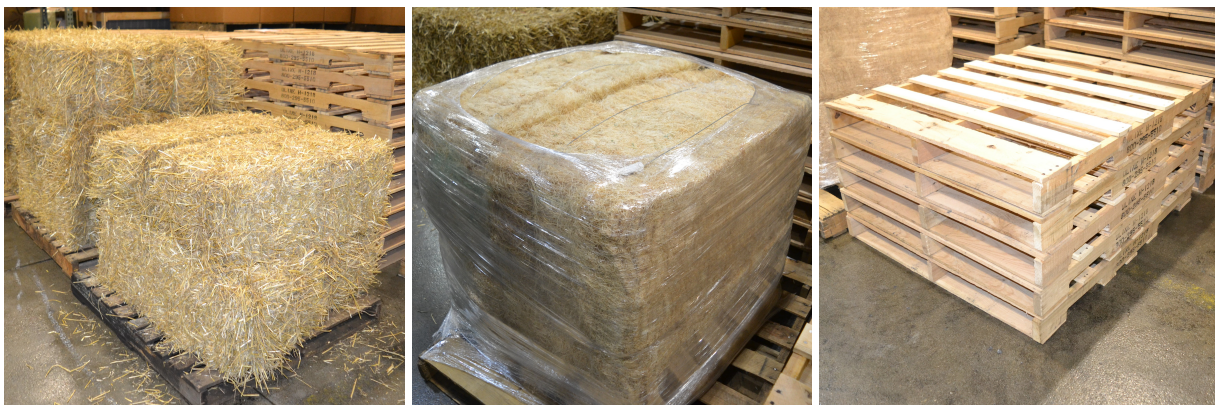
Figure 4.2: Images of straw (left), excelsior (middle), and pallets (right) used for HRR experiments.
