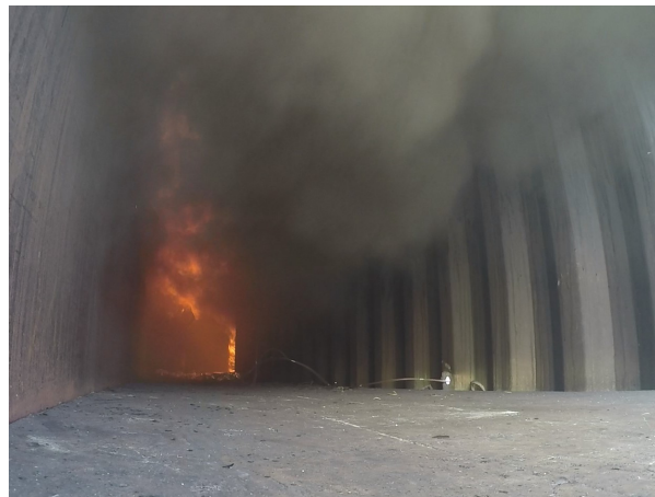
Figure 5.13: Burning in hallway for Experiment 19 (MDF)
