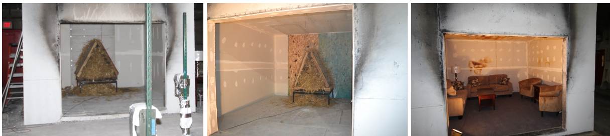
Figure 4.30: Training fuel load position for pallets (left) and OSB (center) and furniture locations (right) for compartment HRR experiments.
