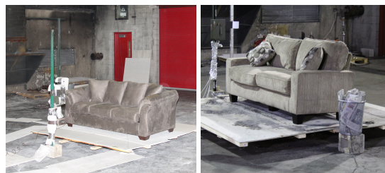
Figure 4.24: Images of the two sofas evaluated in HRR testing. The upholstered sofa (left) and the kit sofa (right). The kit sofa required assembly, whereas the upholstered sofa was delivered in one piece.
